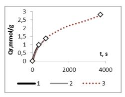
Fig.1. Kinetic curves of specific ozone absorption by aspen wood.
